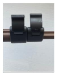
Step 1: Open the catches and extend the stand to the desired height. Close catches to secure height, all 3 legs must be at the same height.
